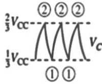
Figure-3: Charging-Discharging of Capacitor of a 555 Timer in Astable Mode
